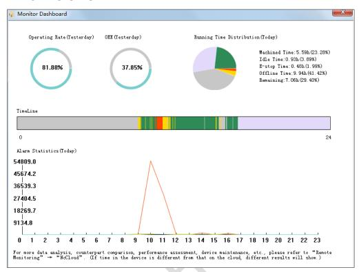
The timeline in the dialog box is set to check the running status of machine tools at all periods of the whole day.
