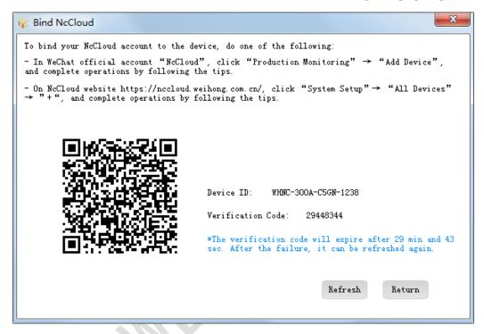
The information of the current CNC system shows in the dialog box, including the QR code, device ID and verification code.
