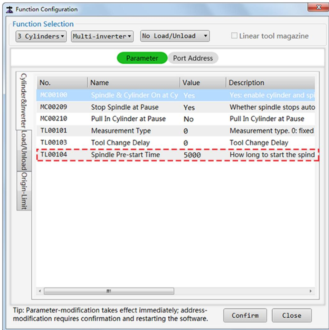
3. Choose numbers of cylinders and inverters, according to actual mechanical structure.
