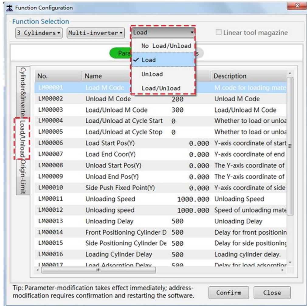
2. Select **Load/unload** in the left of the parameter list and check load/unload related codes:
