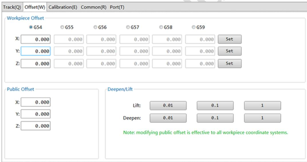
3. To set the workpiece offset, do the following:
