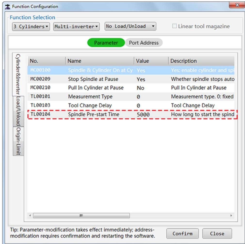
3. Select functions in **Function Selection** area and ensure the selected cylinder combination belongs to multi-cylinder-multi-inverter.
