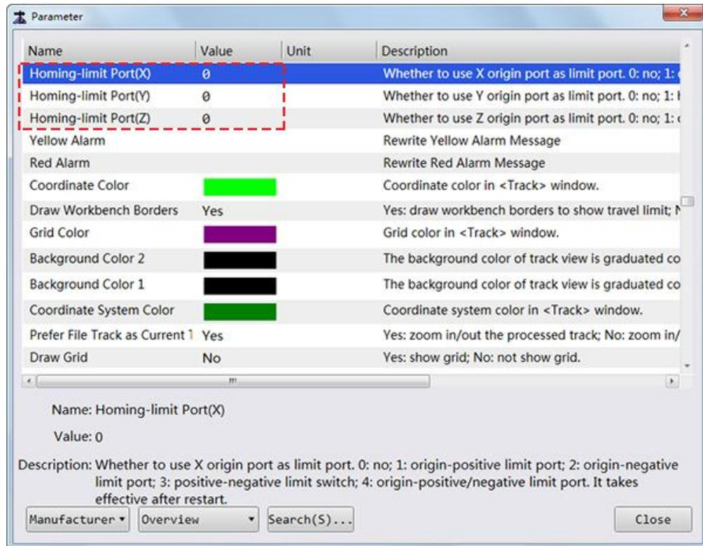
3. Select the axis, its origin and limit switch and modify their parameter settings:
